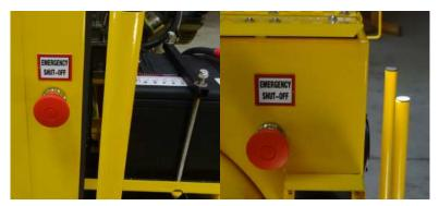
On the older model of heater it was possible for fuel delivery to continue to the combustion chamber in the absence of flame - now the cds "photo" sensor monitors and controls fuel delivery to ensure safe operation at all times. The heater is now CSA, UL, and O-TL certified. On newer models an emergency shut-off switch has been
