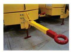
The BT400 NEX features the standard "long bar" and now we offer an optional swivel wheel kit for ease of maneuverability (below right). Tires have been standardized on all models to use tubeless tires and solid rims which are easier to maintain.
