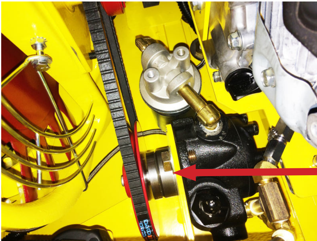
Figure 5-3 V-Belt & Fuel Pump Adjustment
